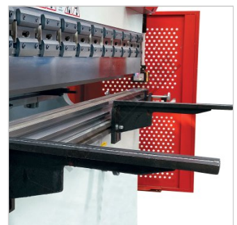
Adjustable Sliding Front Sheet Supports
