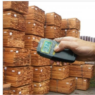
Measuring Moisture Content in Wood
