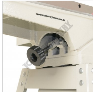
Out-Feed Table Height Adjustment Dial
