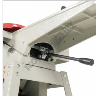
In-Feed Table Height Adjustment
