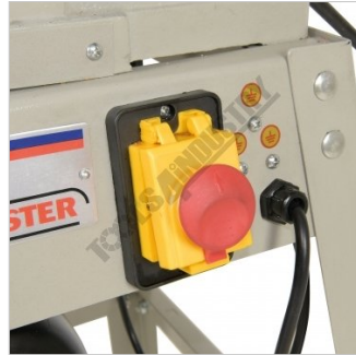
Safety DOL On/Off Switch
