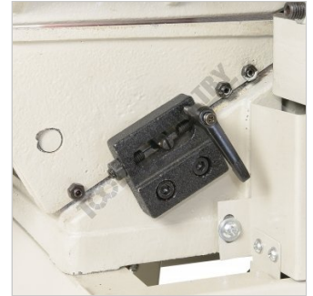
In-Feed Table Height Stop Setting
