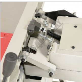
Fence Tilt Mechanism
