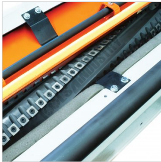
4 x Spiral Cutter Head with Carbide Inserts
