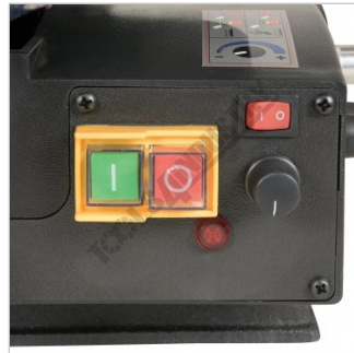
On Off Switch & Variable Blade Speed Dial
