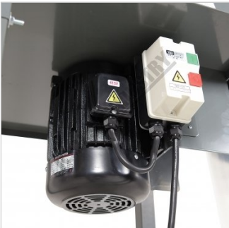
17" Impeller Driven By 5hp 415V Motor
