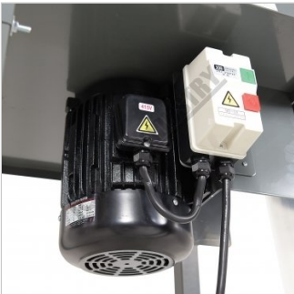
17" Impeller Driven By 5hp 415V Motor
