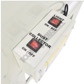
Switches for Light and Dust Collector
