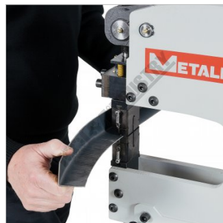
Shrinking Dies In Action 2mm Mild Steel
