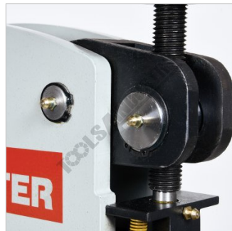
Head Pivot Points with Grease Nipples
