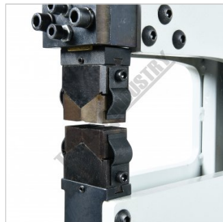
Stretching Dies Shown on Machine
