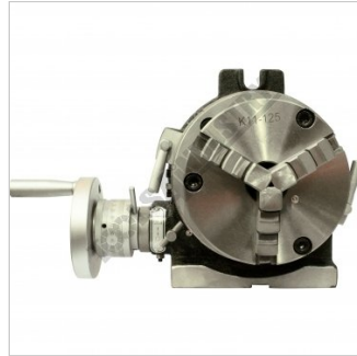
3 Jaw Chuck Fitted in Horizontal Position
