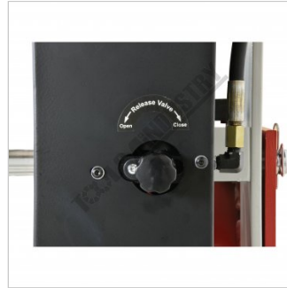
Release valve for hydraulic pump
