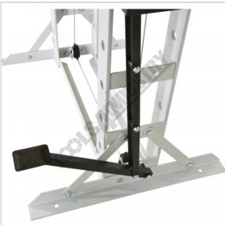
Foot pedal for hydraulic pump
