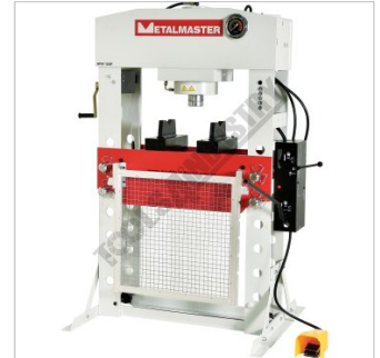
Guard in Down Position Fitted on Press
