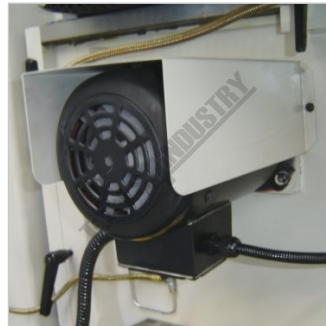
Knee Elevating Motor for Z Axis
