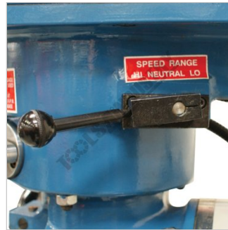
Hi Low Spindle Speed Range Selector
