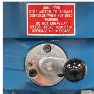
Feed Engage Disengage Drive
