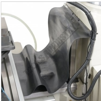
Rear Slideway Protection Cover
