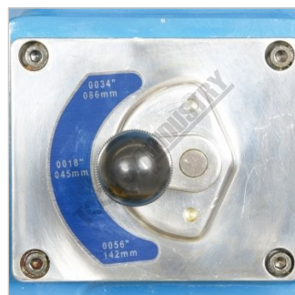
Feed Speed Selector Lever
