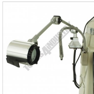
Halogen Worklight and Coolant Hose
