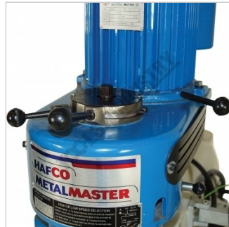
Spindle Brake Lever, High or Low Speed Selector and Belt Tension Lever
