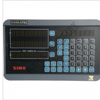
3 Axis DRO with X and Y Axis Scales
