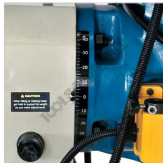
Tilting Mill Head Left & Right to 90 Degrees
