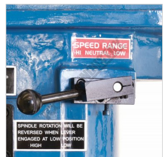
High Low Spindle Speed Gear Lever
