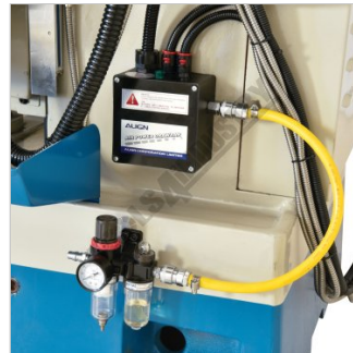
Air Powered Draw Bar System
