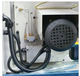
Oil Feeder Distribution Block
