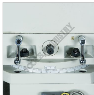
Adjustable Swivel and Sliding Ram
