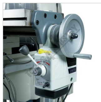
X Axis Power Feed with Rapid
