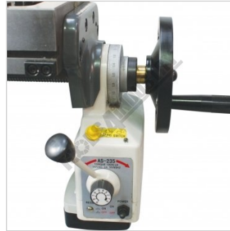
X Axis Power Feed with Rapid
