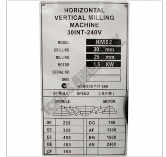
Spindle Speed Chart
