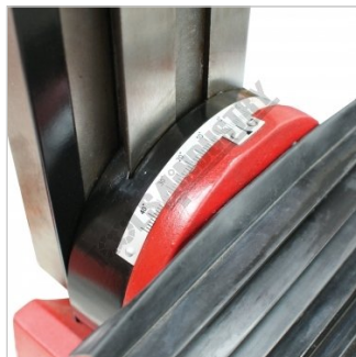
Milling head Tilts 45 Degrees both directions
