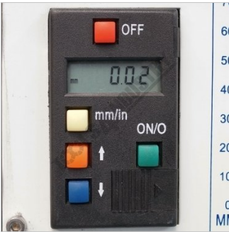
Digital Readout On Quill Depth
