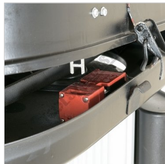
Safety Micro Switch on Belt Guard
