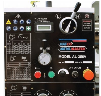
Spindle Speed Controls
