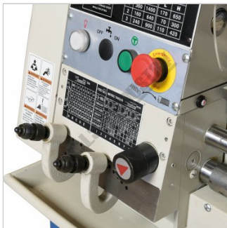
Feed Threading Levers and Control Panel
