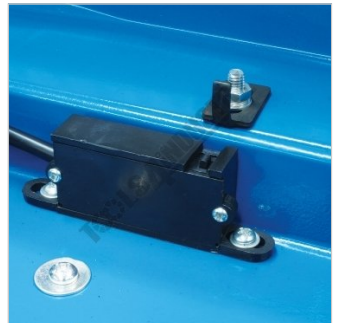
Safety Micro Switch on Pulley Guard
