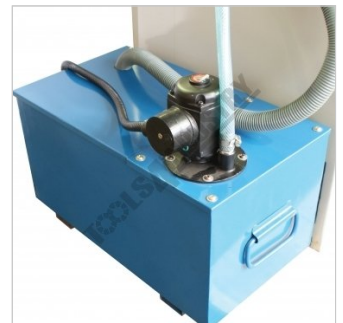
Coolant Pump & Tank
