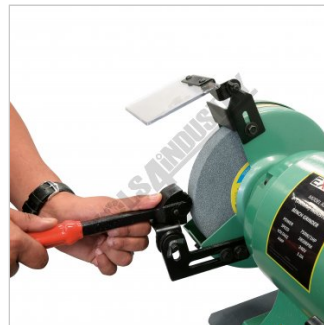
Setup for Dressing a Grinding Wheel
