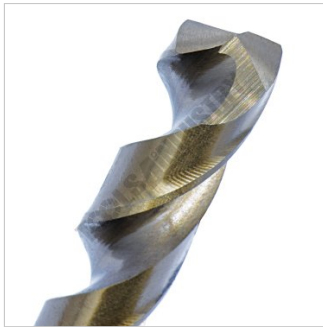
135 Degree Split Point M35 Grade HSS 5% Cobalt
