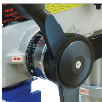
Drilling Depth Stop Setting With Scale
