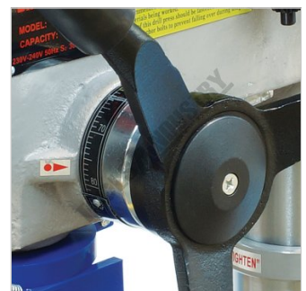
Drilling Depth Stop Setting With Scale
