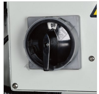
Main Isolation Switch
