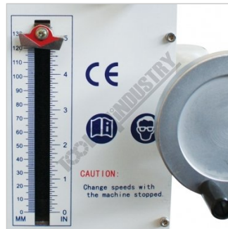
Adjustable Accurate Depth Setting For Increased Productivity
