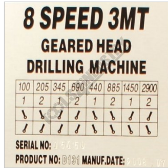
8 Drilling Speeds From 100 2900rpm
