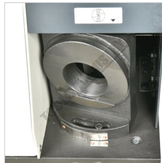
Drill Angle Setting at 90 Degrees
