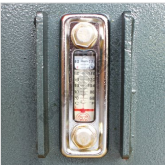
Hydraulic Oil Level Gauge
