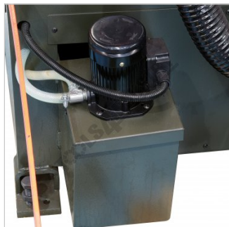
Coolant Pump and Tank
