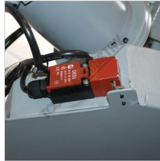
Safety Blade Guard Micro Switch
