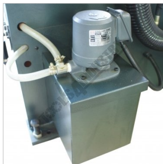
Coolant Pump and Tank
