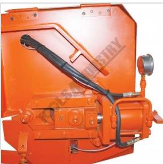
Hydraulic Blade Tension Device Side View
