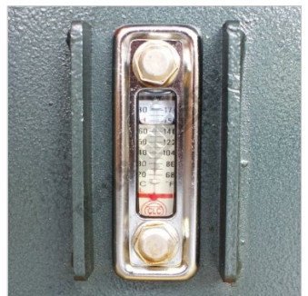
Hydraulic Oil Level Gauge
