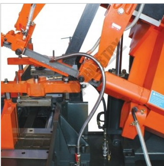
Coolant Nozzle and Fixed Hose Direct Above Blade
