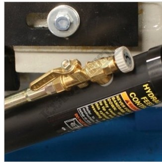
Hydraulic Ram Down Feed Control
