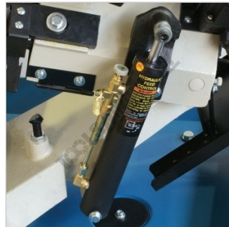
Hydraulic Ram for Cutting Feed Rate
