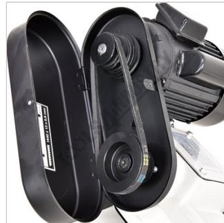
3 Speed Pulley Drive System
