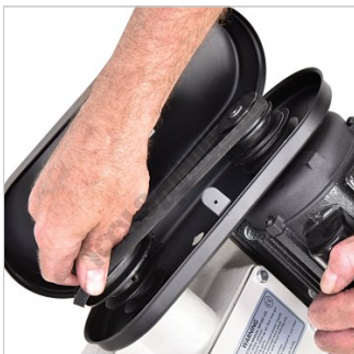
Changing Belt Pulley Speed
