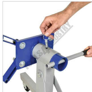
Quick Release-Index Pin for Rotation
