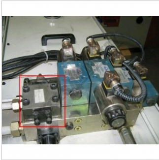
4HS9507 PILOT CHECK VALVE.2
